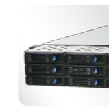
Front accessible modular HDD cage (12 x 3.5 HDD)
