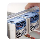
Easy-assembly and anti-vibration fan bar
